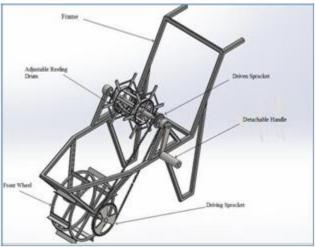
Fig.4 Solid Works CAD Model
